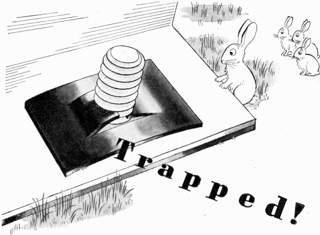
WHEN the 'jaws' of a Spire Nut grip the thread of a bolt, there's no letting go. The whole assembly is held fast—as though a trap had been sprung. And indeed that is exactly what does happen. A Spire Nut tightens and locks itself, biting hard on the bolt thread. Send us along the details (parts or drawings) on any light assembly job, and we'll see if Spire could make a better, simpler, quicker job of it.
