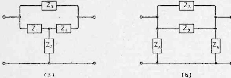
Fig. 4. The original bridged-T circuit (a) can be rearranged to the form of (b) by the usual star-delta transformation.
