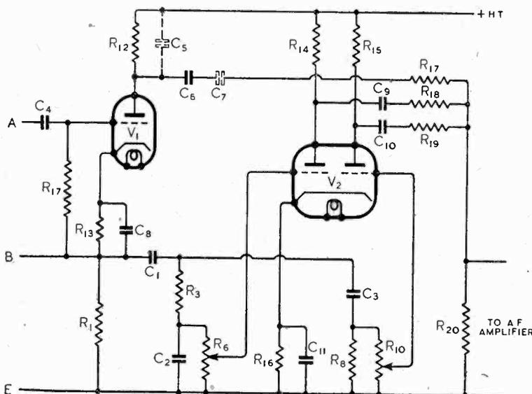
Fig. 12. Circuit of the complete tone control unit.
