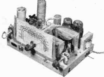
Aluminium screened coils, excellent short wave reception (the special coils used in this circuit give a performance equal to a superhet), 4½ watts output, complete with loud-speaker, all parts, wiring and theoretical diagram—nothing extra to purchase. Chassis dim.: 12in. x 8in. x 6in. to top of dial. 200/250 v. A.C.
