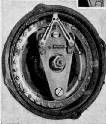
3 in. in diameter is a notable achievement. Although extremely fine gauge wire has to be used, precautions are taken in manufacture to prevent any lateral movement of the turns by the friction of the moving contact.
