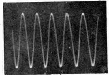
Fig. 16. Oscillogram of the output at 50 c/s. with the bass tone control at maximum and the treble tone control at minimum.
