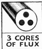
Three Cores of Flux ensure flux continuity. No lengths without flux are wasted. Consistent high quality joints are obtained with comparatively unskilled labour. Exactly the correct proportions of solder to flux are provided. Separate fluxing operations are obviated and no extra flux is required. The three cores of flux being evenly distributed over the cross section of the solder provide thinner
