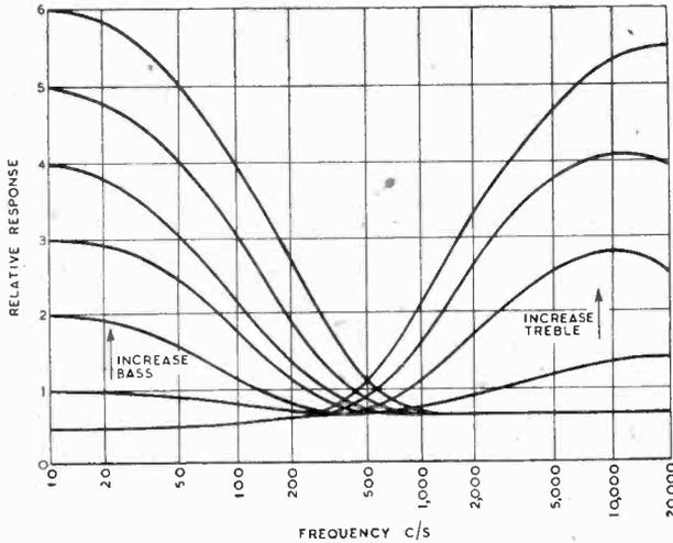
Fig. 13. Experimental results obtained from the circuit as shown in Fig. 12, omitting condensers  $C_5$  and  $C_7$ . The "increase bass" readings were taken with the treble tone control at minimum and the "increase treble" readings with the bass tone control at minimum.
