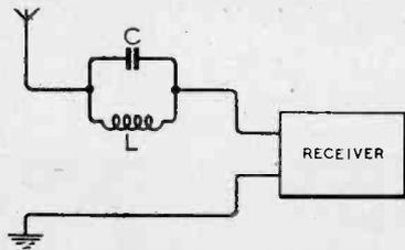
Fig. 1. Conventional wavetrapp circuit text-book device, although actually it is a simple and practical circuit.
